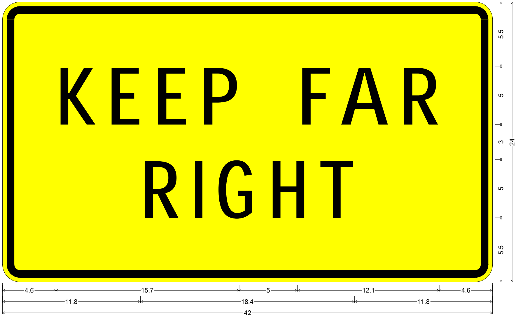
W16-14: KEEP FAR RIGHT (PLAQUE) Note: Only to be used with a W11-1: Bicycle Sign; 1.5" Radius, 0.6" Border, 0.4" Indent, Black on Yellow; "KEEP FAR" D; "RIGHT" D;
